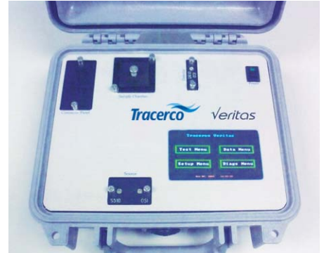
Figure 2 – Tracerco's UV/VIS spectrometer used to analyze produced water samples.
