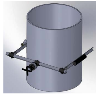
Illustration of a TRACERCO Diagnostics™ FMI yoke system positioned across the member under inspection.
