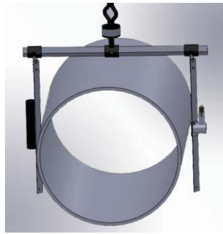
Illustration of a TRACERCO Diagnostics™ FMI yoke system positioned across the member under inspection.
