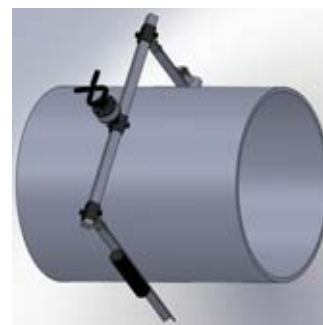
Figure 4 – Example of Pipe Scan Set-up
