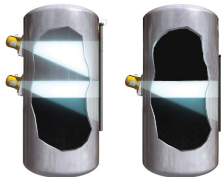
Figure 7 External source variation for bulk level control, alarm and critical process shutdown.
