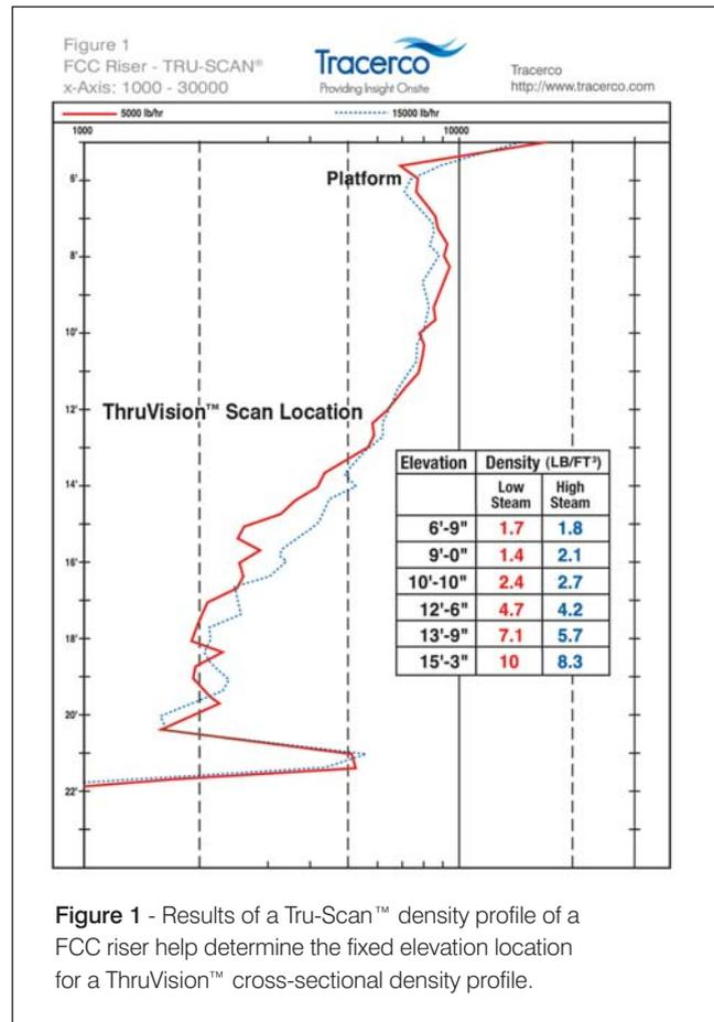
Figure 1 - Results of a Tru-Scan™ density profile of a FCC riser help determine the fixed elevation location for a ThruVision™ cross-sectional density profile.
