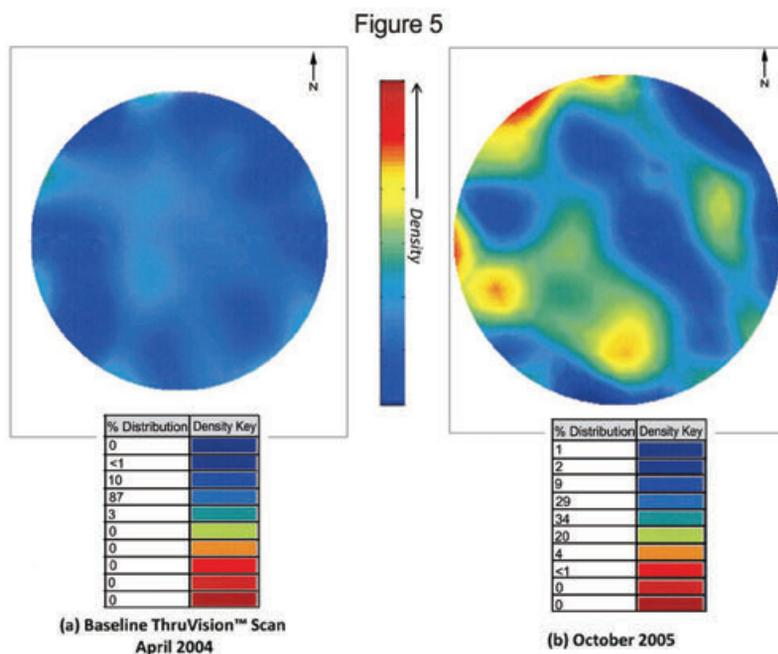
Figure 5 – (a) Baseline scan results of crude vacuum tower wash bed; (b) ThruVision™ scan result at the end of Cycle 1.
