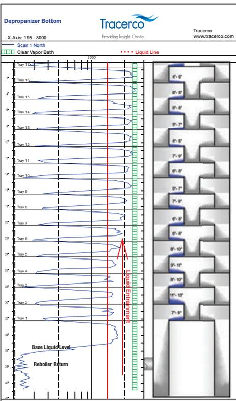
Figure 8 – Tru-Scan™ results decided the course of action for the refinery during their turnaround. Modifications to the tower were made instead of preparing to replace damaged trays which scan results found were not necessary.
