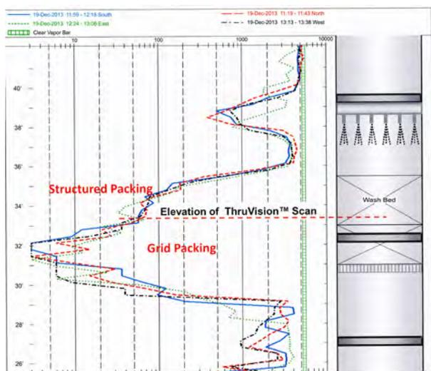
**Figure 3.** Baseline Tru-Grid™ scan results of a crude vacuum tower. The four scan lines matched, indicating the same process density along each scan line, suggesting good liquid distribution. One can see the shift in radiation counts, from right to left, due to the heavier bulk density of the grid packing.
