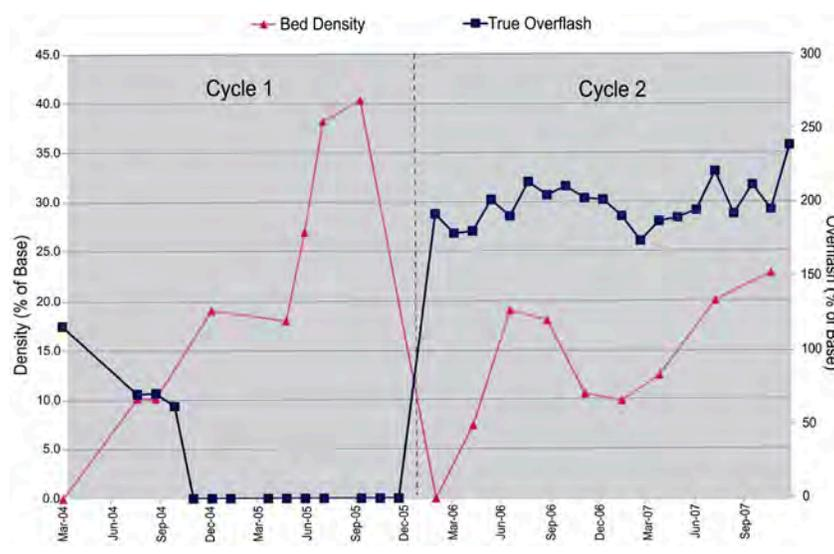
**Figure 9.** Wash bed packing density vs true overflash.
