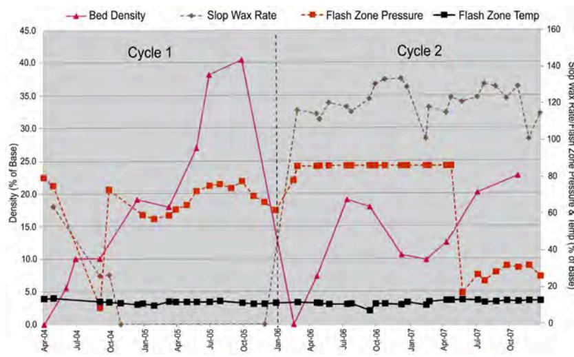
**Figure 8.** Wash bed packing density vs slop wax rate, flash zone pressure and flash zone temperature.
