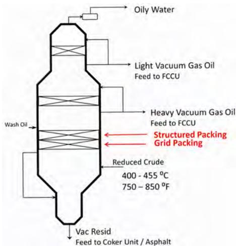
**Figure 1.** General process diagram of crude vacuum tower.
