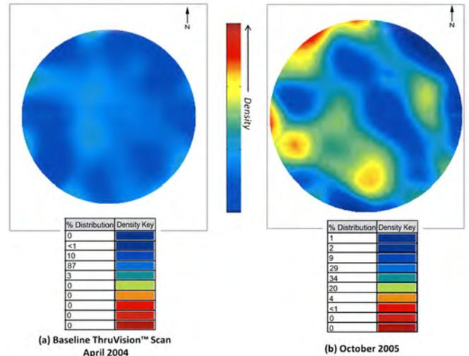
**Figure 4.** (a) Baseline scan results of crude vacuum tower wash bed; (b) scan result at the end of Cycle 1.
