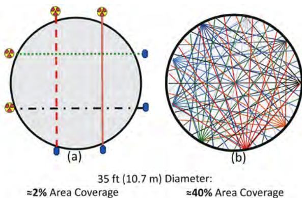
**Figure 2.** (a) A 4-way grid scan typically used to scan the entire height of the tower for troubleshooting; (b) a tomography scan completed at one elevation for a detailed cross-sectional density profile.
