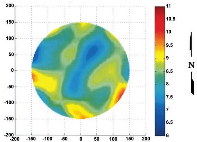
Figure 3 The second set of results at low rates revealed a higher degree of poor liquid distribution (900 gpm wash oil rate).
