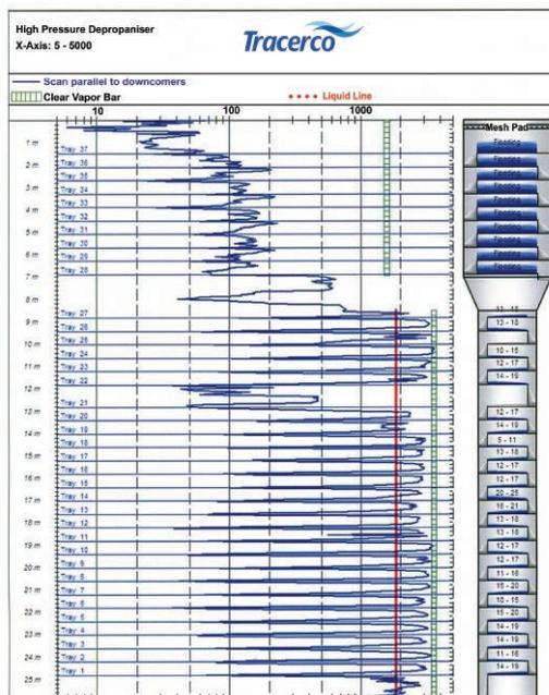
Figure 7 – Initial scan showed that flooding started at Tray 28.
