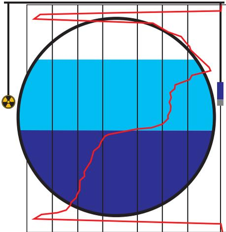
Figure 11 – In this case the Slug Catcher pipe was filled with two possibly three phases: fouling (solids), liquid and gas.
