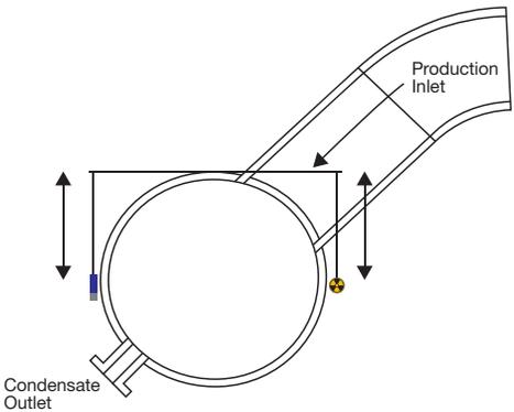
Figure 12 – Due to the possible different material segregations, the pipe scan was performed as a 'slice' scan (scanning vertically through the Slug Catcher).
