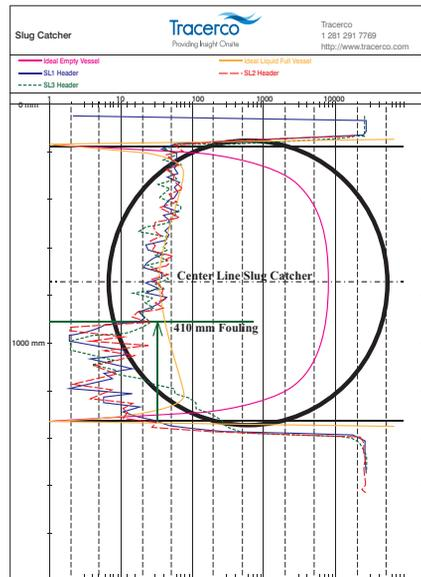
Figure 14 – Results at the three scan locations of the Slug Catcher including the idealistic results of an empty pipe.
