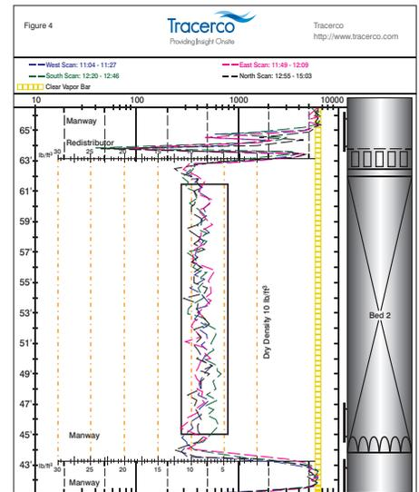
Figure 4 – Typical grid scan results through a packed bed including the patent pending PackView™ liquid retention scale overlaid on the scan data.
