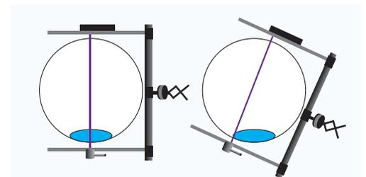
Figure 10 – Suspect sections of pipe will be tested at 2 or more different orientations to provide diameter measurements and determine the deposit layer.
