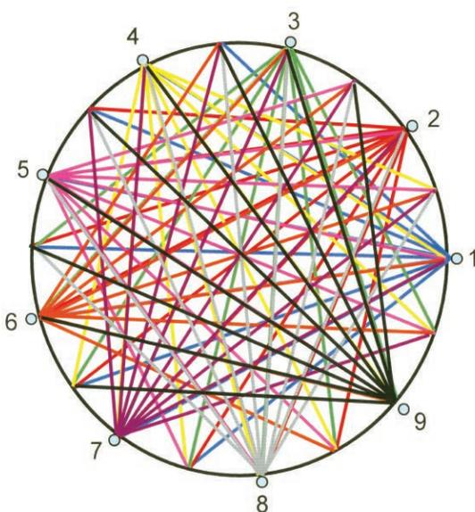
Figure 17 – A Tracerco™ ThruVision scan uses multiple scan chords at the same elevation. In this case study a 9x9 scanning pattern was used.
