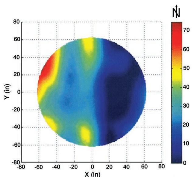
Figure 18 – Scan results showed a higher than expected density on the western half and a lower than expected density on the eastern half of the mist eliminator pad.
