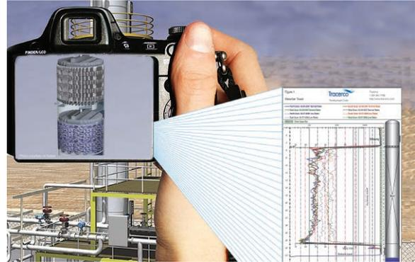
The last issue of Tracerco Insight (Vol 6 Ed 1) featured our patent pending FrothView™ technology illustrating how using Tracerco's new measurement detector technology and analysis of gamma scan data provides quantitative information about the useful capacity of trayed towers. In this article you will learn how applying this technology to packed towers can determine the % liquid fraction providing a measure of the maximum useful capacity of the packing.
