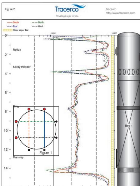
Figures 1 & 2 – Grid Scan orientation and a typical example of scan results illustrating good liquid distribution.
