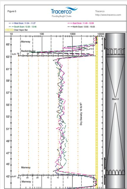
Figure 5 – Scan results shown from Figure 3 with the liquid retention scale included indicating how “bad” the liquid mal-distribution was at the time of the scan.
