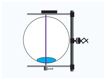
Figure 9 – Illustration of a gamma scan orientation for long sections of horizontal pipe containing primarily a one phase flow.
