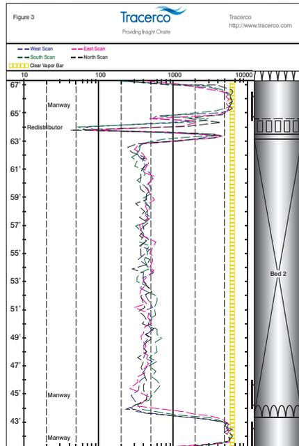
Figure 3 – Grid scan results implying mal-distribution, but the question is what is the quantity of liquid mal-distribution?
