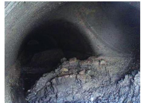
Figure 15 – Internal photo showing a view of the extent of fouling within the Slug Catcher.
