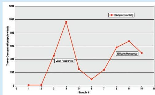
a leak and effluent response. The minimum calculated leak based on the laboratory analysis was measured at 0.2%. Analysis of the results narrowed the leak to a specific heat exchanger bank. The application of the chemical tracer technology saved the plant a significant amount of maintenance costs by narrowing the leak to a specific bank, minimising production down time.
