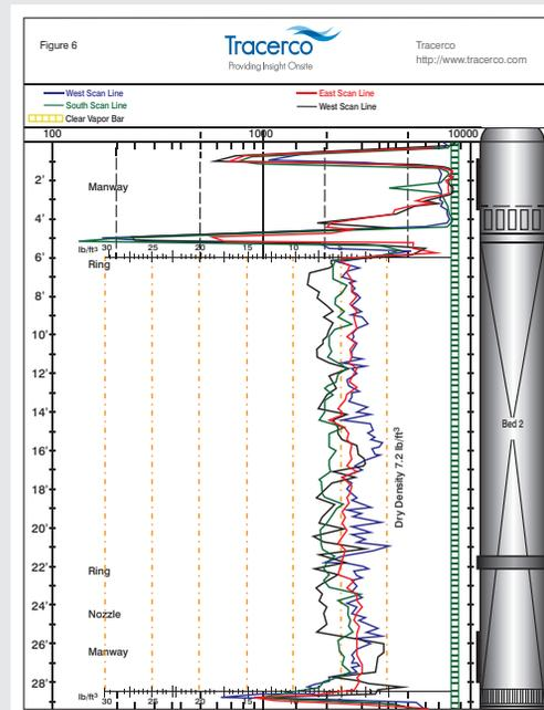
Figure 6 – An example of liquid mal-distribution where the liquid retention scale indicates a relatively large difference in liquid density representing a significant liquid mal-distribution.
