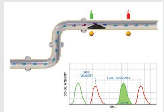
Figure 16 – Tracerco's slug monitoring system provides slug flow characteristics to allow operations the ability to control and suppress vapor or liquid slugs.
