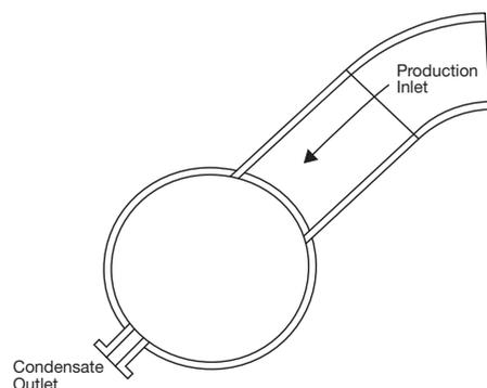
Figure 7 – Illustration of Slug Catcher design.
