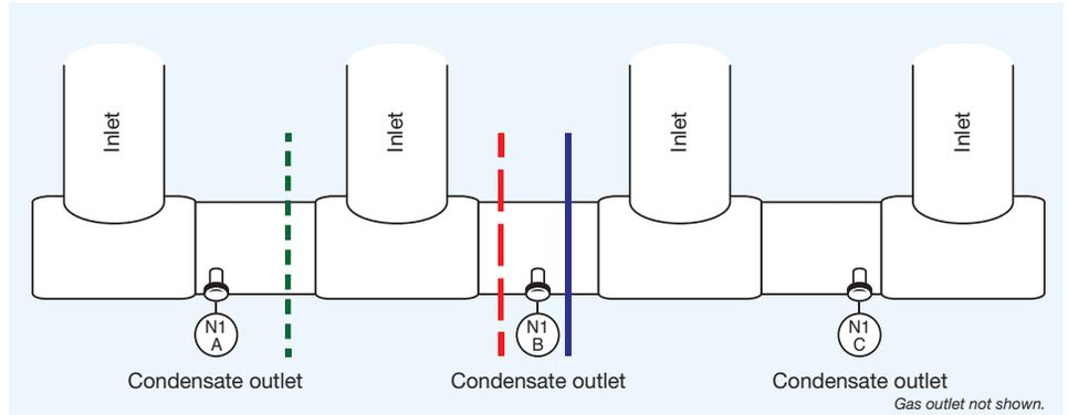
Figure 8 – Pipe scans were performed at 3 locations on the Slug Catcher to determine the cause of level control problems in the pipe.
