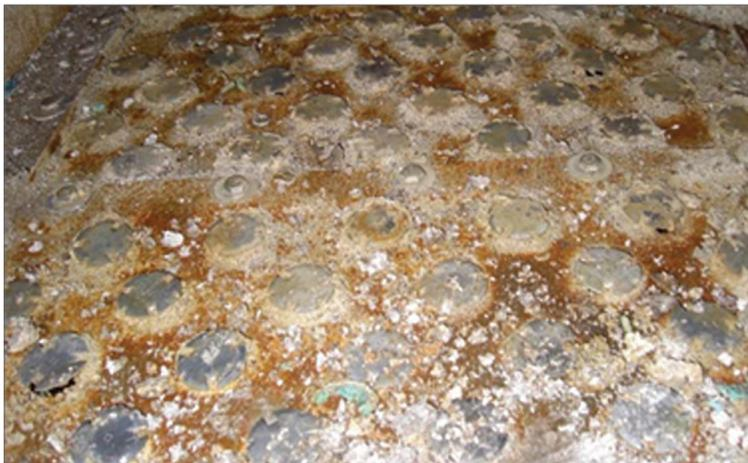
Figure 7 Active area of Tray 1 showing polymer plugging the valve units
