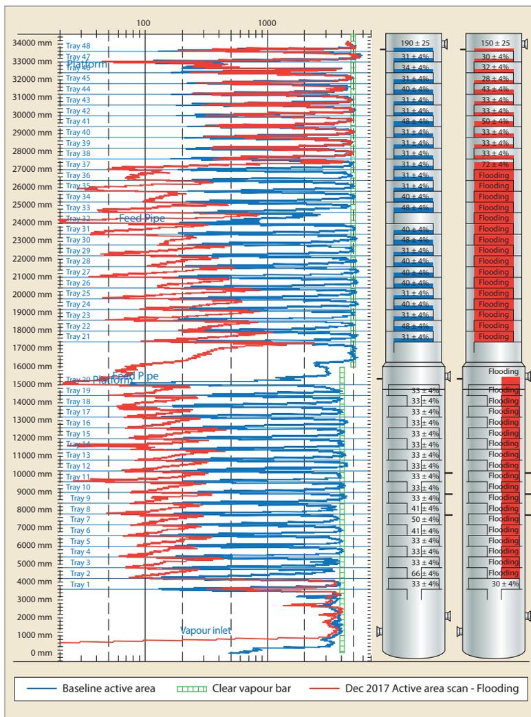
**Figure 5** December 2017 scan of tray active areas under flooding operating conditions. Blue curve is the baseline scan; red curve shows flooding started at Tray 2 and had propagated up the column to Tray 38
