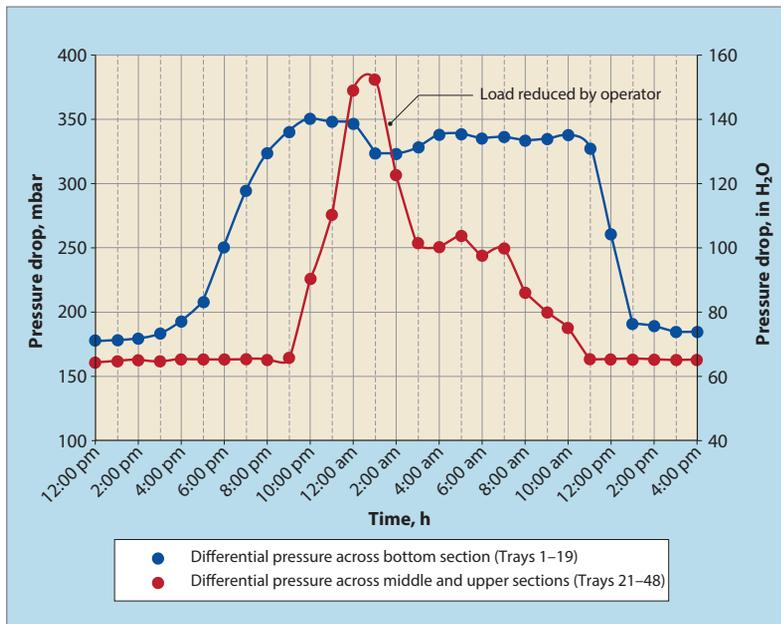
Figure 2 Differential pressure measured 4-6 October 2017 (courtesy of Linde AG)
