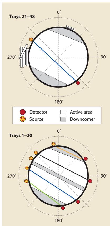
**Figure 3** Scanline orientations: August 2017 baseline and December 2017 flooding scan – blue scanline; December 2017 east active area and downcomer scans at normal conditions – black, orange and green scanlines
