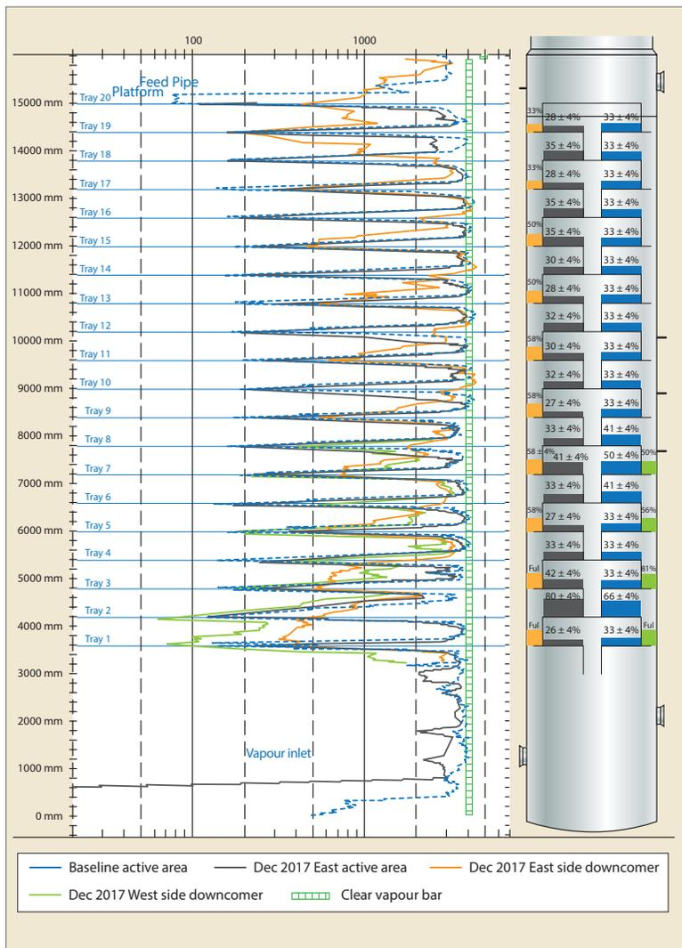
**Figure 6** December 2017 scans of two-pass tray eastern active areas (black data curve), east side outside downcomers (green data curve) and west side outside downcomers (orange data curve) at normal operating conditions. Original two-pass western active area baseline scan data shown by dashed blue curve
