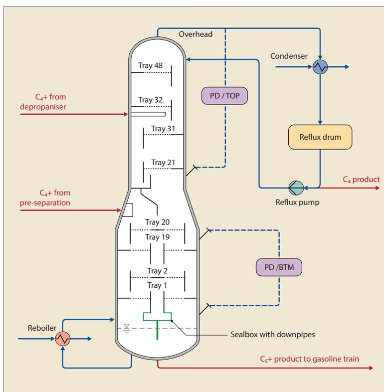
Figure 1 Simplified process scheme of the debutaniser (courtesy of Linde AG)
